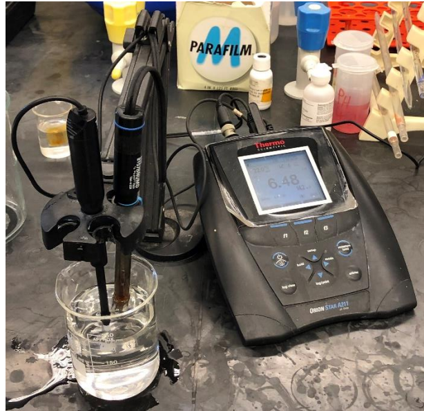
Figure 5.8: Digital pH meter
