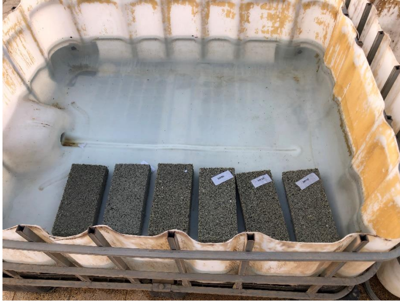
Figure 5.26: Water Absorption test
